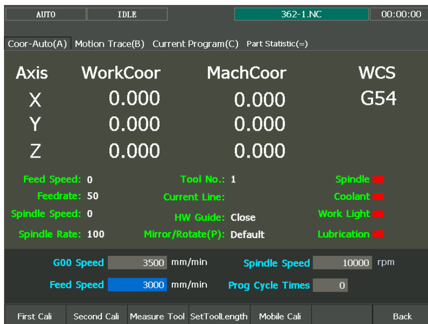
Fig. 3-16 Sub-screen of tool calibration
