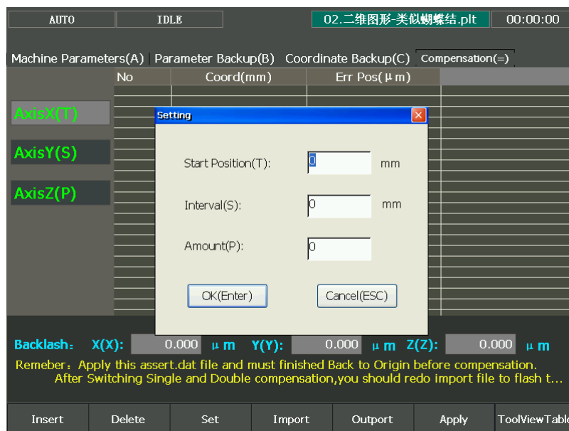
Fig. 3-37 Compensation parameters setting
